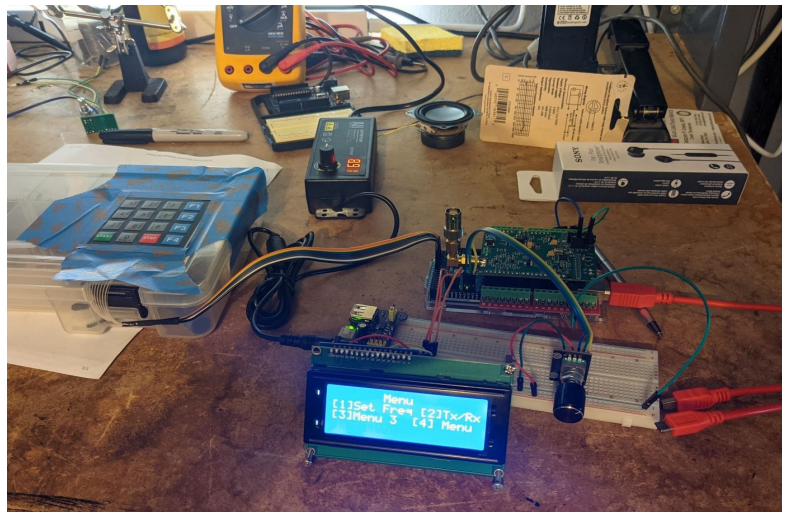
Shown above is Greg Cheng - KC3SMW's Homebrew ArduHamCeiver. An example of how useful Arduino can be to the Ham Radio Amateur.
