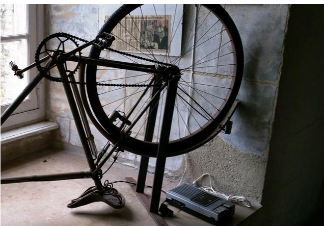
This bike was used to generate power for a small radio by the Resistance. Being caught meant certain death. He demonstrated by turning the pedals which made the tape recorder play.
